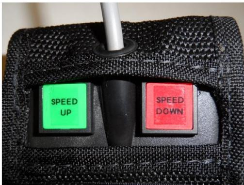
box, the rider can then adjust speed(s) by pressing the SPEED UP or SPEED DOWN buttons located top of the remote control pouch. Each press of either button will result in a 10% STEP in speed; with a total number of 10 STEPS available. Cycling power on the Ranch Sorter control box will reset the STEPPER back to center: (-5 steps) center (+5steps)
