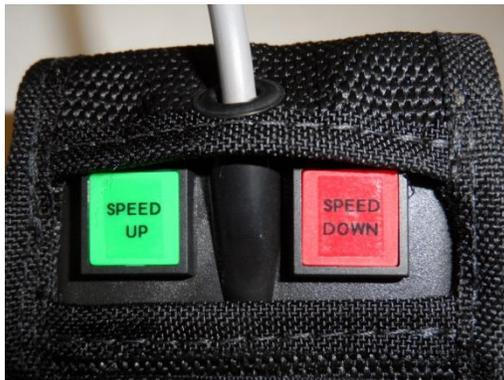
box, the rider can then adjust speed(s) by pressing the SPEED UP or SPEED DOWN buttons located top of the remote control pouch. Each press of either button will result in a 10% STEP in speed; with a total number of 10 STEPS available. Cycling power on the Pro Cutter control box will reset the STEPPER back to center: (-5 steps) center (+5steps)
